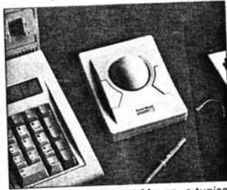
The Kensington Expert Mouse, a typical trackball, has a centrally located ball.
